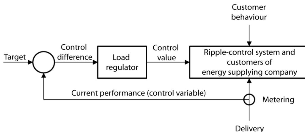
The target is the reference variable. The load regulator calculates the control value (control objects that need to be turned on and off) out of the difference between control variable and reference variable. The ripple control system sends the corresponding ripple control commands to the ripple control receivers which turn the loads on respectively off.
